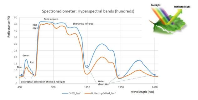
**Figure 1:** Typical reflectance profile of plants showing absorption of light in the blue and red bands (450-500 nm; 625-740 nm), and reflection of light in the green (500-560 nm), Near Infrared (760-1200 nm) and Infrared bands (1200 nm +).
