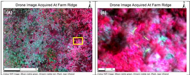
**Figure 5:** False colour infrared image of the 4 band multispectral data by Parrot Sequoia at Farm Ridge in KNP (panel A). The zoomed-in imagery at the right (panel B) shows an area with Orange Hawkweed plants marked by the yellow sticks.
