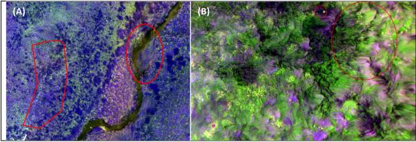
**Figure 6:** (*A*) Tearing of the processed mosaic image acquired using 3DR Solo Drone and Parrot Sequoia sensor (processed in Pix4D). Errors were spotted in the highlighted areas. (B) Wavy patination likely caused by insufficient image overlap.
