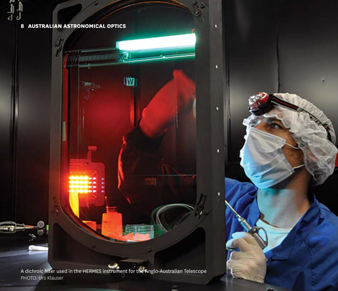
A dichroic filter used in the HERMES instrument for the Anglo-Australian Telescope
