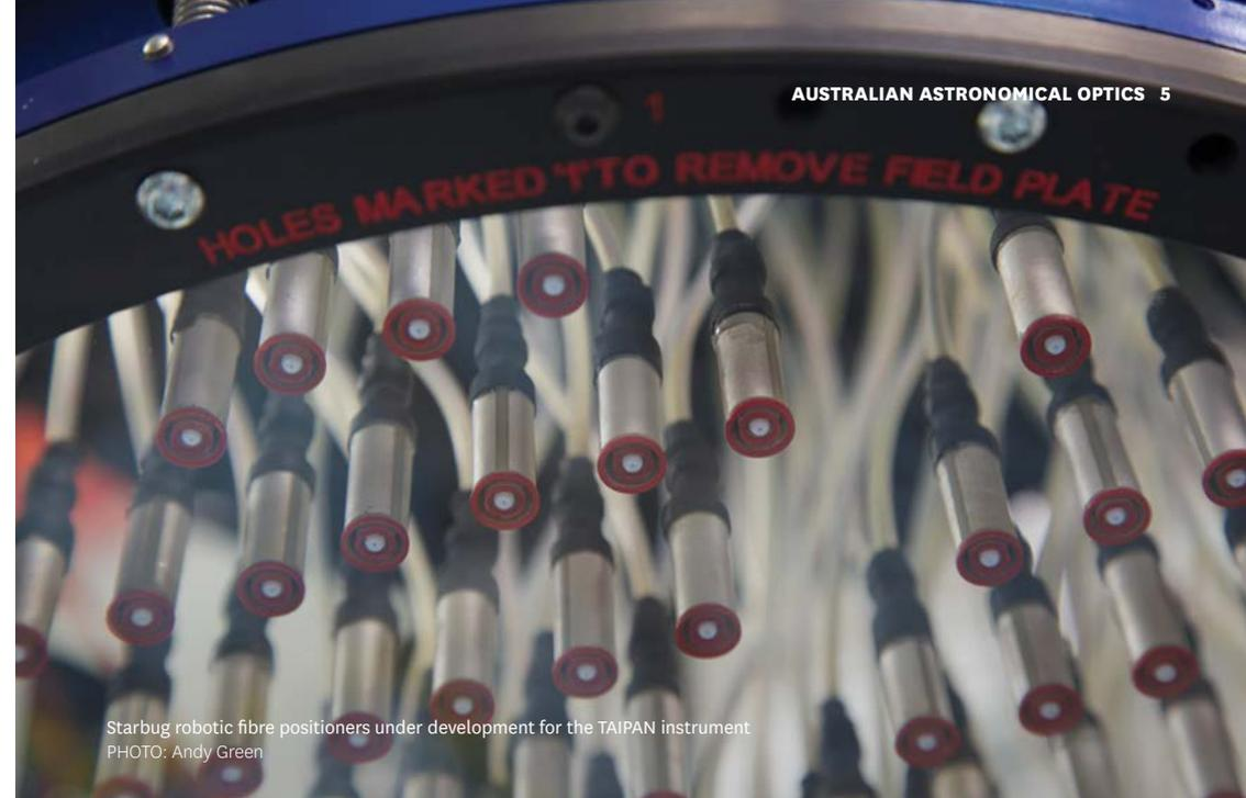
Starbug robotic fibre positioners under development for the TAIPAN instrument
