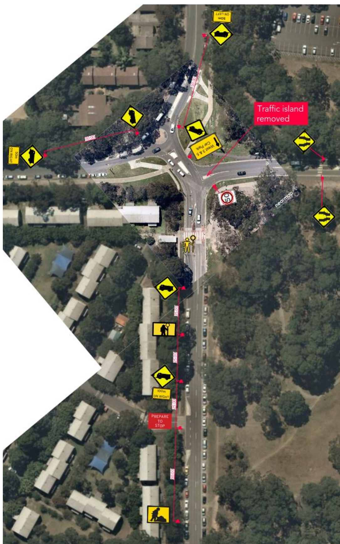
Figure 27 – Traffic Control Plan – Culloden Road and Gymnasium Road (CTMP-006)
