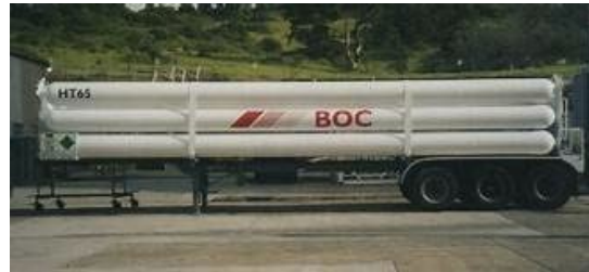
Typical Type I, transportable tube trailer
