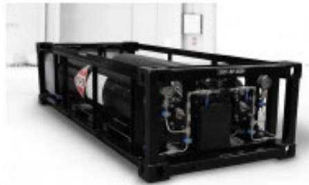
Typical modular Type IV, 950bar static storage (e.g. Hexagon)
