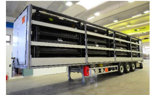
Typical Type III tanks, bundle
