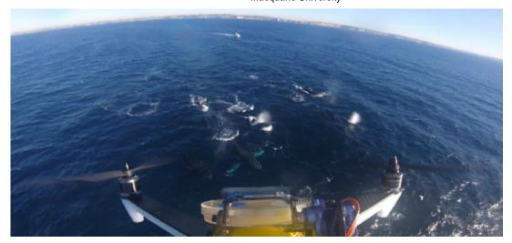
Biological Sciences researchers have led the design and construction of a new system to sample whale microbiota—the combination of natural bacterial colonies that live in an organism—by flying over and collecting exhaled vapours from their blowholes.
