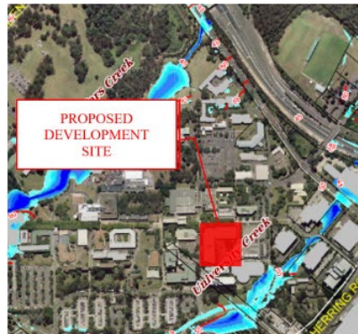
Excerpt from 100 Year ARI Flood Map from Macquarie Park Floodplain Risk Management Study & Plan by Bewsher (2010)
