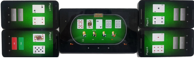
Fig. 6. TexasHoldem: App is installed and launched only in the center (local) device where BoardActivity is currently being executed. Four remote devices in both sides are executing PlayerActivity with different cards each other.
