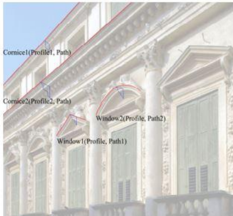
Figure 4. Two groups of components sharing the same path and profile in Palazzo Barbaran da Porto
